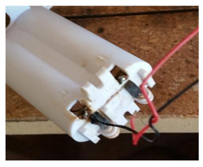
So you can try to resolder the leads but the wires used are so tiny it can be difficult. I replaced the leads with 22 awg stranded wire. Stranded is required because the pads on the circuit board are very small
