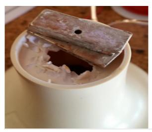
the sensor glued inside. There are 3 steel blocks in the base for ballast which I removed. I extended the leads with 22 awg stranded wire and fished it through the heatshrink tube.
