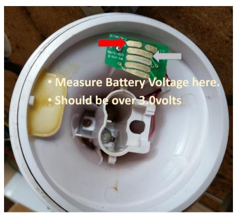
If the battery voltage is low or non-existent; remove the battery holder with two screws.
