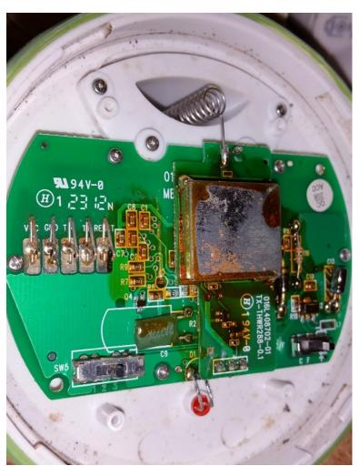
significant that part was so I replaced the diode from a nonworking temp sensor.
