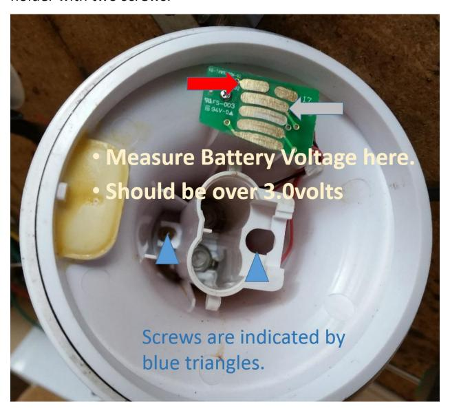
The most common problem I have found is broken or corroded leads to the battery holder.
