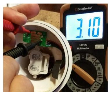
If you measure 3 volts you can try the sensor again. Notice I used the via holes to probe.
