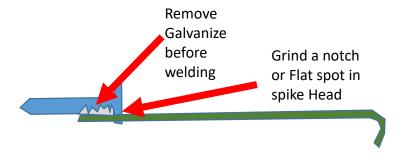
galvanization from the spike before welding the rod. Welding on Galvanization is reported to generate poisonous gases. I used a plumber's torch to heat the non-welded end of the steel Rod to bend it round for safety. I use a steel hose clamp and Zip ties to secure the Polypro tube to the stakes. I use a lot of zip ties and I usually buy them at Harbor Freight on Sale.
