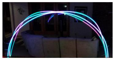
I run/fish the WS2811 strip lights (12v) through the tubing. I make all the strip LEDs face the same direction. I use the standard JST connector on the WS2811 strips which *fit through the tube*. The WS2811 strip lights come with
