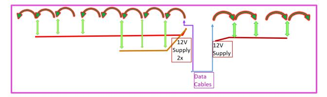
Figure 1 Power Lines shown with Power injection into Arches and Data Cables
